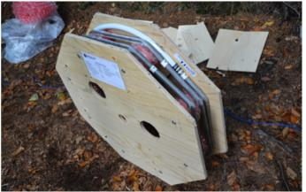
Fig.3 - 6 meters long SAA sensor (20 segments)
