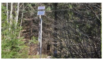
Fig.4 - Solar panels that supply the datalogger through battery
